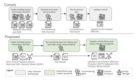
Figure 5. Functional Testing to Commission Controls Process
