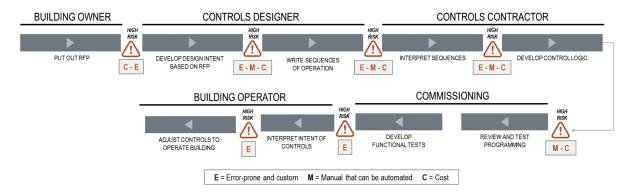
Figure 1: Conventional control delivery workflow (Paliaga et al., 2020)
